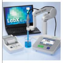
Upon endpointing SevenCompact<sup>™</sup> allows multiple archiving options: the data can be stored, printed or transferred to LabX direct. Any combination of these three options is possible giving you total flexibility.
